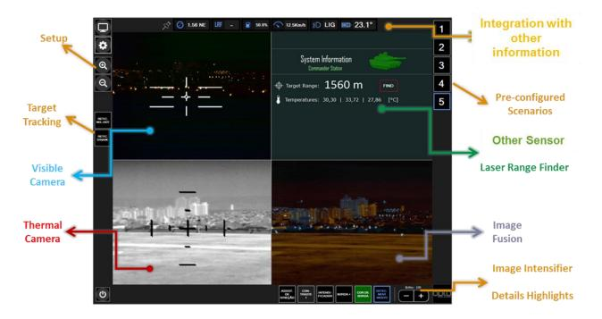
Different crosshair, colors and highlights can be chosen. Other data can be read and processed with the obtained target distance. Algorithms like edge highlighting and motion detection are used to improve capacity.
