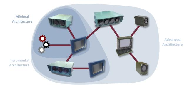
Due to its modularity, the architecture has the capability to remain operational even with a damaged sensor box.
